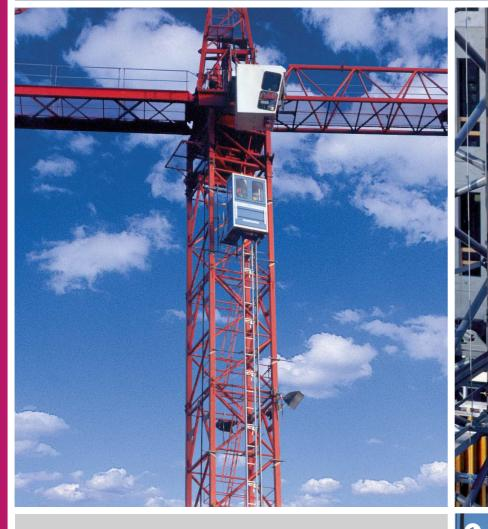
The GEDA 2 PK is an individually applicable rack and pinion hoist with aluminium ladder sections. It is able to transport the crane operator to his working place in very short time. Its big advantage: concentrated working from the beginning regardless of meteorological conditions and motivation. The GEDA 2 PK meets the requirements of the European Machinery Directive.
